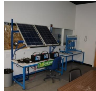
Figure L. Solar photovoltaic panels in Room 119 at the Betz Technology Center are set up at a student work station for the Renewable Energies Technology program.
